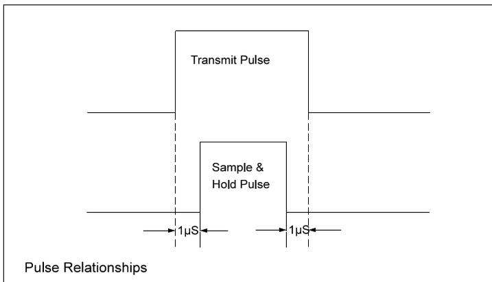
This loss of sensitivity can largely be recovered using a sample and hold circuit between the IF output of the unit and the amplifier. The sample and hold circuit would typically consist of a FET series switch turned on when the oscillator is turned on, and a shunt capacitor which is then charged from the IF output of the
