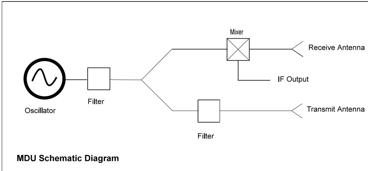
One of these signals is further filtered and feeds the transmit antennas of the unit, illuminating the volume to be protected. The other signal is fed to the local oscillator input of a balanced mixer as the reference signal against which the Doppler return signal is compared.
